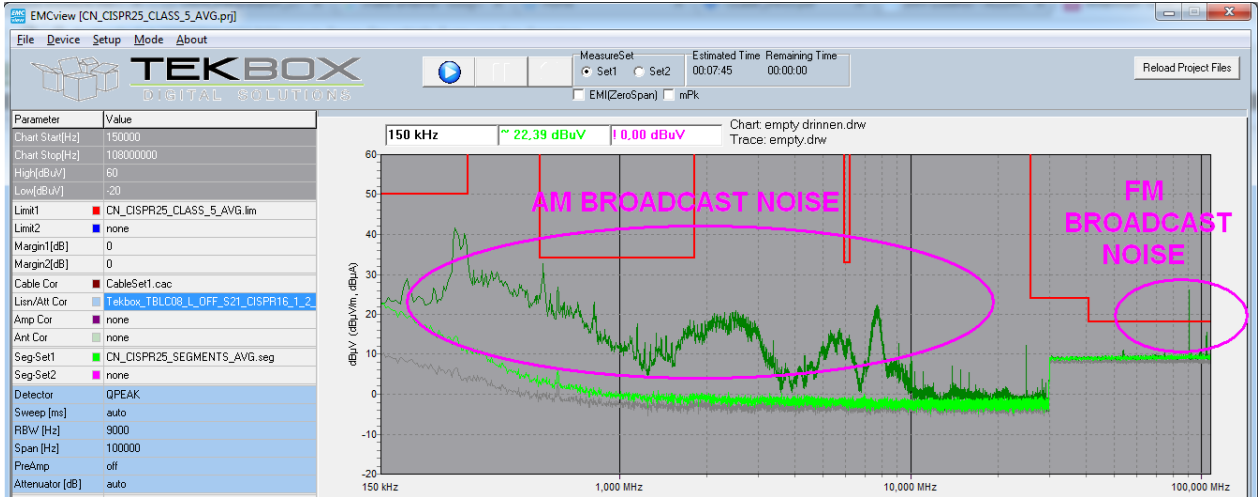
Picture 5: CISPR 25 conducted noise measurement; DUT not powered
